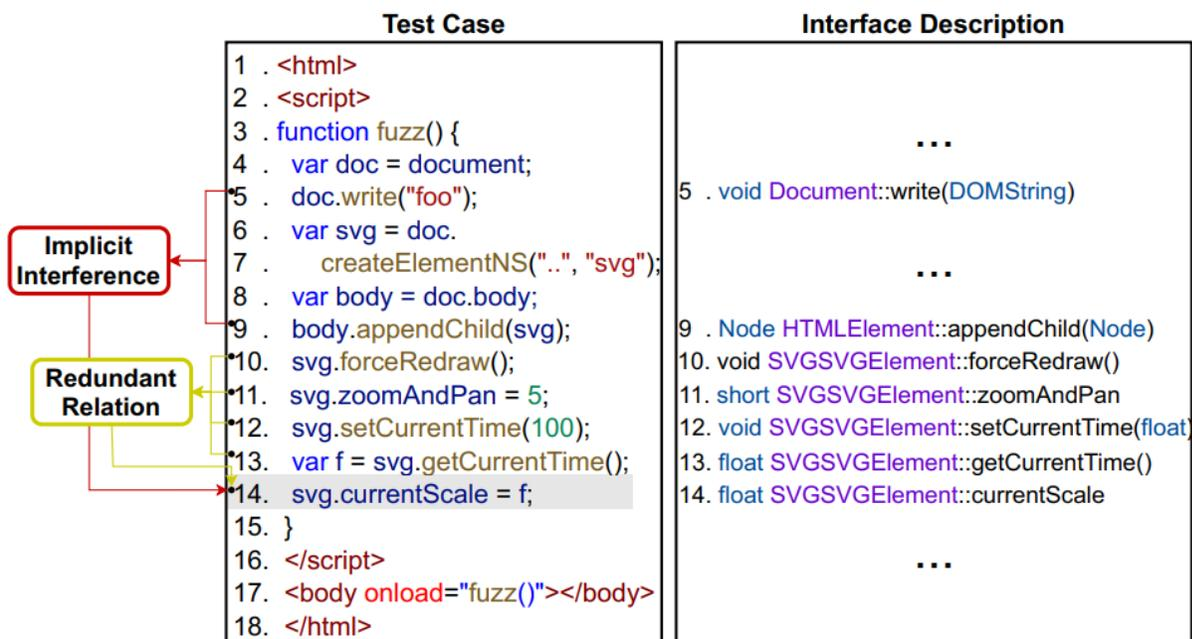
(a) A test case and its corresponding interface descriptions
